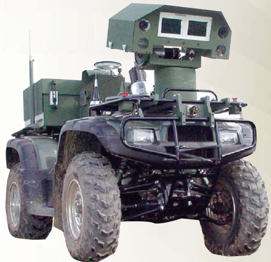
Figure 3: The unmanned vehicle used for AVOSCET validation: DARPA's PerceptOR vehicle
